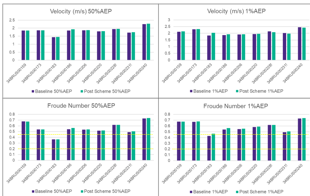
Apx Figure 9: Brusna (Glenree) Cross Sections – channel velocity and Froude number comparisons
